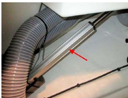
Electrical piston Location: Cockpit locker
