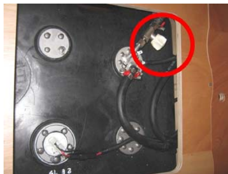
Fuel supply valve Location: On the fuel tank
