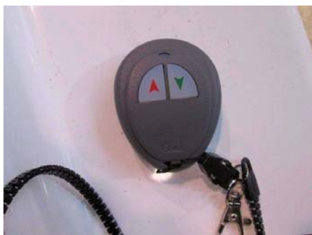
Control - Aft platform Location: Port cockpit (under the gas cylinder locker cover)
