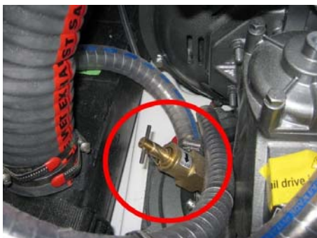
Engine water intake valve: Located directly on the saildrive Access: Port cabin
