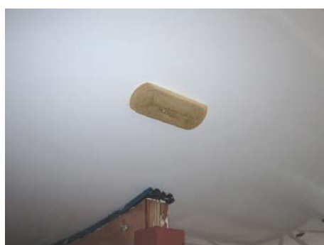
Condenser (Microbead plate) Location: Hanging locker - Starboard aft cabin
