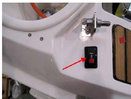
Control - Aft platform Location: Port cockpit (under the gas cylinder locker cover)
