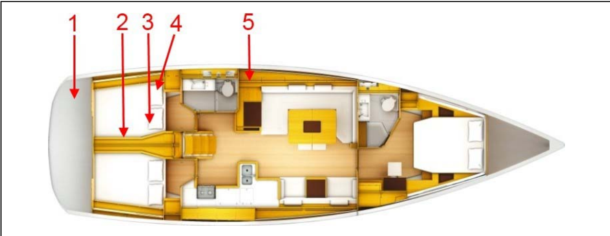
Ref 1: Heater Access: Port cockpit locker
