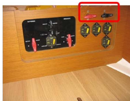
Ref 4: Generator battery switch (Positive & Negative terminal)
