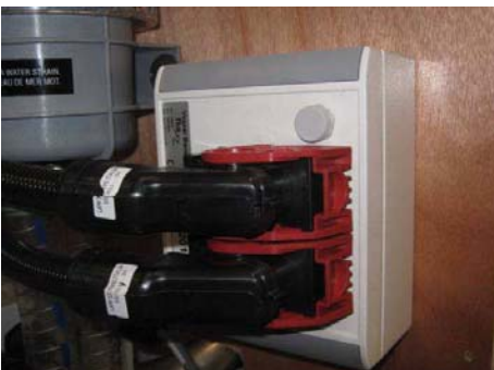
VMU housing (Vessel Management Unit) (Ref 6)
