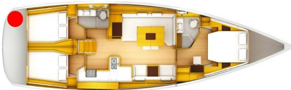
Extinguisher access hole Access: Port cockpit locker
